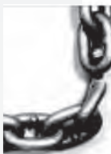
Broken & Worn Links
